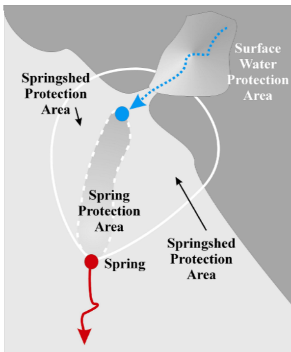
Figure 2 - Hypothetical spring protection zones in a scarp-bounded springshed.
