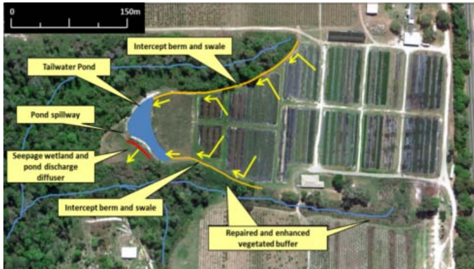
Figure 4-9. BMP modifications to surface discharge from overhead irrigation area. Post implementation, overland flow is intercepted by intercept berms and direct via a swale to a tailwater pond. Water detained in pond is released at a controlled rate to a seepage wetland and eventually flows back to the tributary.
