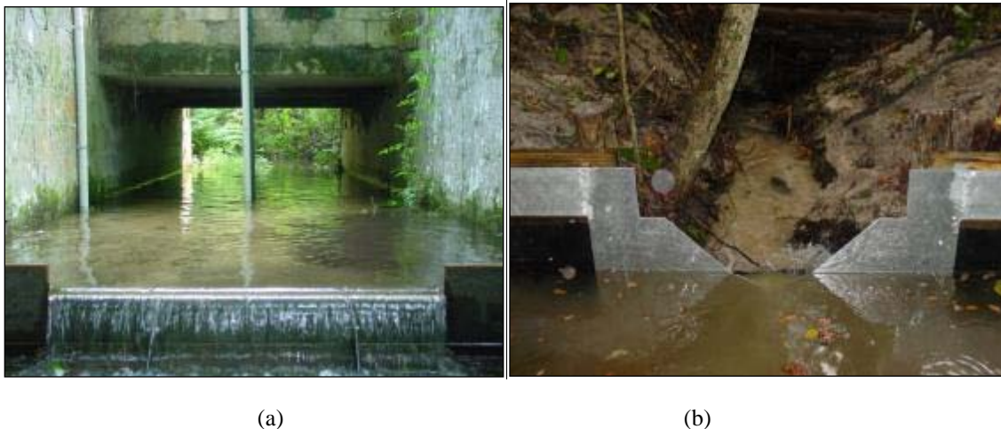
Figure B1-1. Example of two weirs being used to measure surface flows, a) rectangular weir, and b) compound “V-notch” weir.
