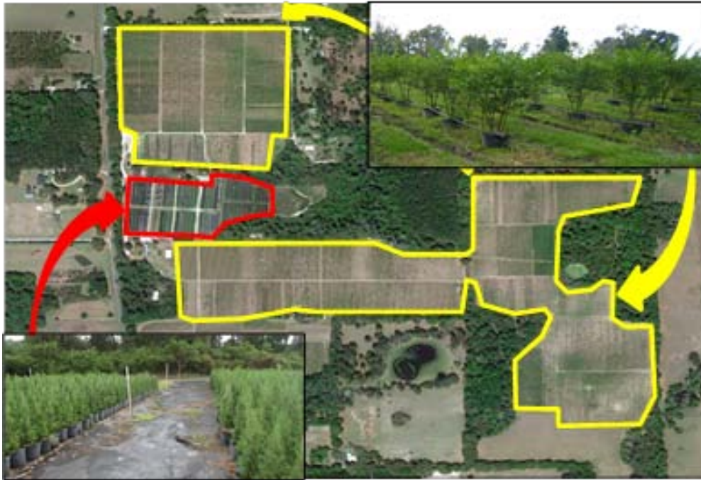
Layout of nursery showing irrigated areas using overhead irrigation (red) and those areas using microirrigation (yellow)
