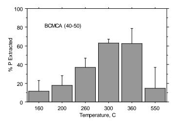
**Figure 16.** Effect of temperature on P extraction. Mid-depth (40-50 cm) of BCMCA stations included. Error bars represent  $\pm 1$  SD.
