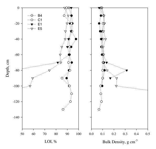
**Figure 8.** Loss on ignition and bulk density of soil samples from WCA2A and BCMCA.
