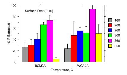
**Figure 21.** A comparison of pyrolysis-extractable P between BCMCA and WCA2 for the surface (0-10 cm) soil depth. Error bars represent  $\pm 1$  SD.
