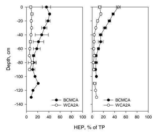
**Figure 12.** Hot water extractable P content of soil samples from BCMCA and WCA2. Error bars represent  $\pm 1$  SD.
