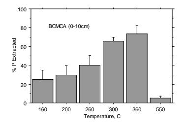
**Figure 15.** Effect of temperature on P extraction. Surface (0-10cm) of BCMCA stations included. Error bars represent ±1 SD.
