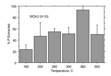
**Figure 18.** Effect of temperature on P extraction of peat samples. Surface (0-10 cm) of WCA2 stations included. Error bars represent  $\pm 1$  SD.
