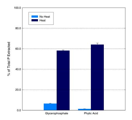
Figure 13. Autoclave extractable P content of glycerophosphate and phytic acid.
