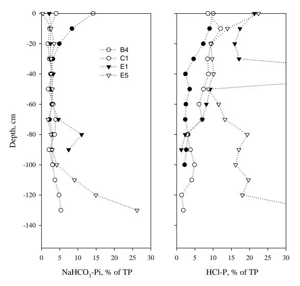
**Figure 10.** Bicarbonate and 1M HCl-extractable P content of soil samples from WCA2A and BCMCA.
