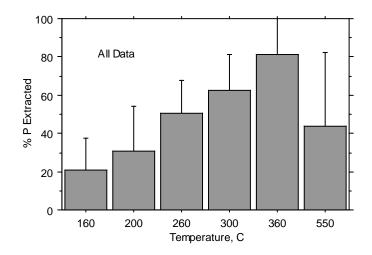
**Figure 14.** Effect of temperature on P extraction. All data (three depth's, two wetlands, four stations) included. Effect of temperature is significant at p< 0.0001. Error bars represent  $\pm 1$  SD.
