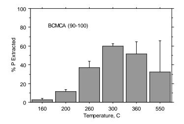
**Figure 17.** Effect of temperature on P extraction of peat samples. Lower depth (90-100 cm) of BCMCA stations included. Error bars represent ±1 SD.
